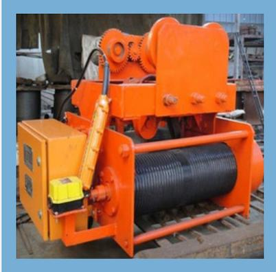
Electric Wire Rope Hoists
